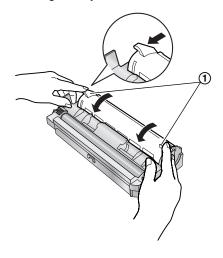
**6** Make sure that the triangles (①) match, to install the toner cartridge correctly.
